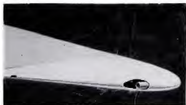
Except for pilot's controls, mechanism is mounted entirely on rotor (diagram, right). The small rocket engine rides inside stream-lined rotor-tip fairing (above). Rocket exhaust, which provides thrust, is practically invisible and almost silent
